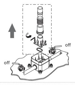
turn off the valve, take out the pipe cleaning spare parts.
