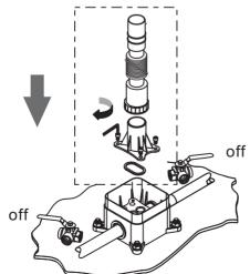
install pipe cleaning spare parts.
