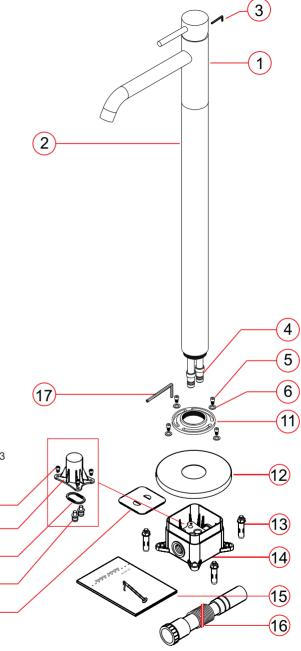
specifications: water pipe thread: G1/2 working pressure: 0.1Mpa~0.5Mpa working temp.: 3°C ~ 85°C working material: normal water producing standard: GB 18148-2003
